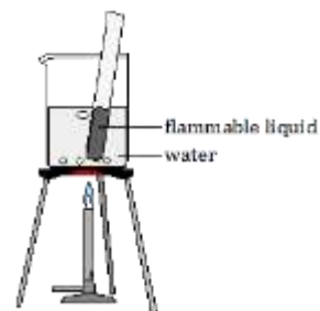
Fig. 2: Heating a flammable liquid
