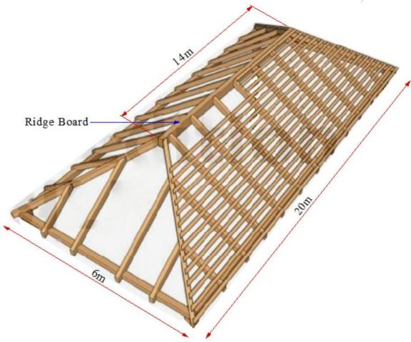
The roof frame has a rectangular base with dimensions of 20 m by 6 m and the ridge board of 14 m centrally placed. The triangular faces are equilateral.
